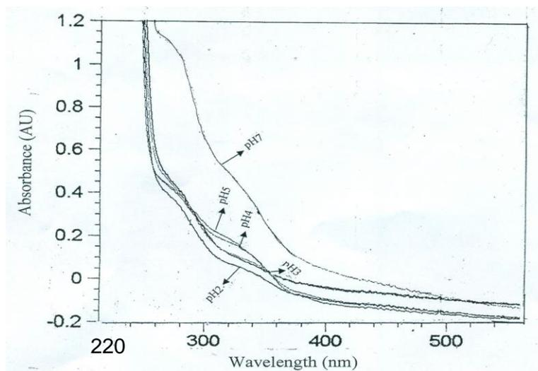
**Figure 2:** UV spectra of [Zn( $\gamma$ -pga)] complex in aqueous solution at different pH.
