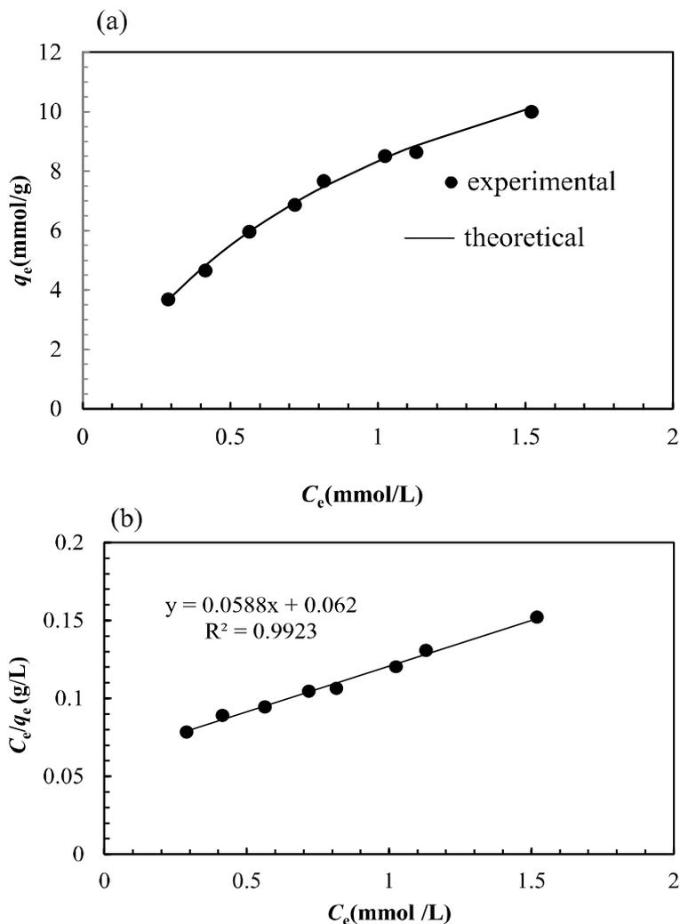
**Figure 4:** Binding isotherm (a) and the corresponding linearized plot (b) for the chelation between Zn(II) ions and  $\gamma$ -pga at pH 5 and temperature 30 °C. The theoretical solid line in Figure 4(a) was generated by using the Langmuir model equation (2) and the values of  $a_L$  (0.94 L/mmol) and  $K_L$  (16.13 L/g) obtained from Figure 4(b).
